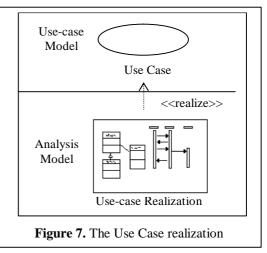
the iteration diagrams specifying the message flows between objects playing the roles in the Collaboration. These diagrams are expected to realize the use case above.
