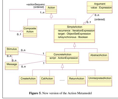
propose to sub classify a SimpleAction in both ConcreteAction and AbstractAction. ConcreteAction will be the superclass of the concrete actions that were defined in the metamodel until now (i.e. CallAction, CreateAction, etc.), while an AbstractAction will specify those actions that will be refined. These new metaclasses improve formality of the Use Case metamodel allowing for the definition of the Use Case refinement hierarchy, as we will see in next section.
