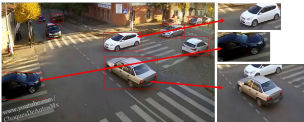
Figure 5: Video extraction for each tracker (car). The left side shows a surveillance video, and the right side shows three small videos, each one generated per car. Each small video has different sizes but all of them have 30 frames.
