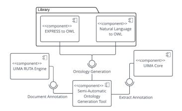
Fig. 3. Proposed Tool Component Diagram
